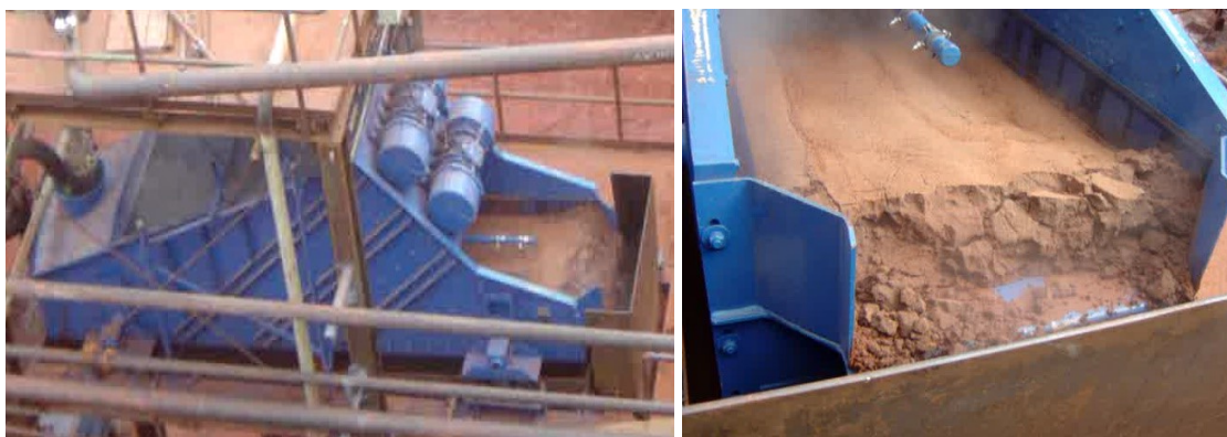
Figure 5. Dewatering screen, discharge of separated and dewatered sand [6].
